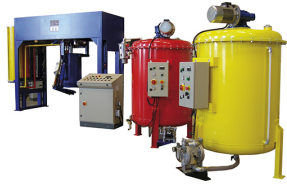
Isolblock batch block plant
